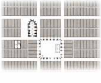
▲ A 1248 plan for the bastide Monpazier, France, shows horizontal alleys bisecting residential blocks.
